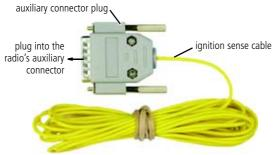
The TMAA04-05 ignition sense kit provides a mating plug for the radio's auxiliary connector. The four metre length of cable from pin 4 of the plug connects to the vehicle's ignition signal.
