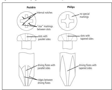
Figure 1.3 Identifying Pozidriv and Philips screws and screwdrivers
