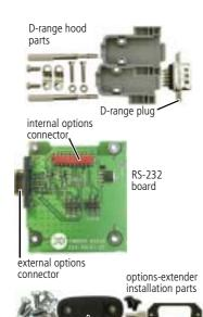
The TMAA01-02 RS-232 board fits inside the radio in the options cavity and is connected to the main PCB by the internal options connector and loom.
