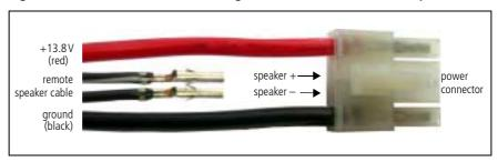
Figure 16.2 Power connector wiring of the TMAA10-06 remote speaker
