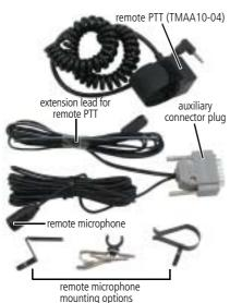
The TMAA10-04 remote PTT kit and the TMAA10-05 hands-free kit plug into the radio's auxiliary connector. Both kits use the remote electret microphone to replace communication through the usual rugged microphone. The rugged microphone can still provide hookswitch operation, if this is required.
