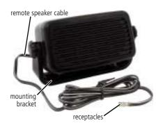
The TMAA10-03 remote speaker (for the 25 W radio) and the TMAA10-06 remote speaker (for the 40 W/50 W radio) are installed in parallel with the radio's existing internal speaker. The remote speaker can then be installed at some distance from the radio, or it can be used to increase the volume of the audio from the radio's existing internal speaker.
