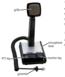
The TMAA10-01 desktop microphone is an omnidirectional dynamic microphone which can be used in dispatch situations, where the microphone is positioned on a flat surface. The desktop microphone plugs into the microphone socket on the radio control head.
